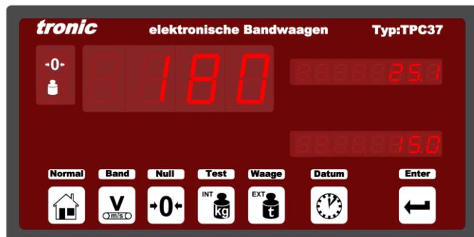
4. Now turn the screw of the left sensor back down so the load cell is loaded again. Adjust the screw that the mainscreen of the TPC37 shows 90.
