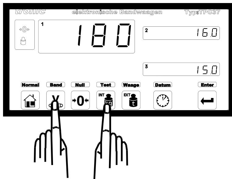
The value on Display 1 schould be between 200 to 220 with no material on the conveyor belt. If this value is not ok please check if there is something wrong at the mechanic.
