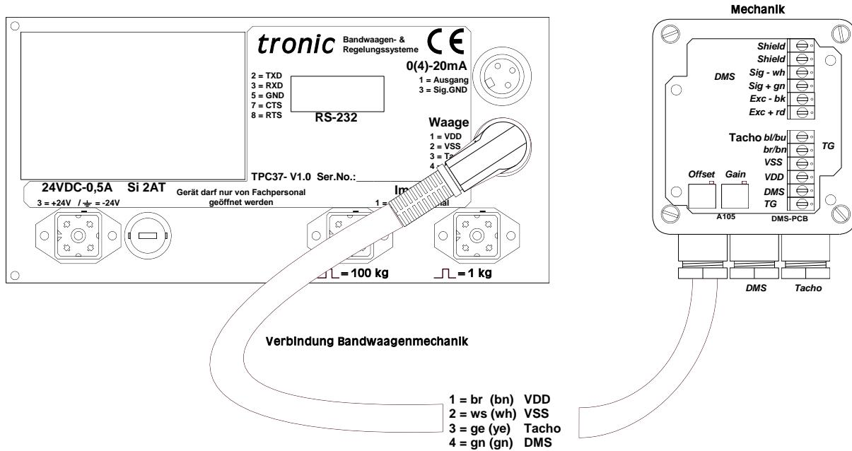
The second Value on Display 2 ist the actual current from the tachogenerator. This value should be about 15.0-17,0 or 24.0-25.5. By turning the wheel of the tachogenerator slowly this 2 states shall be displayed.
